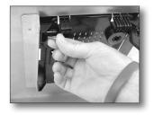
The bolts we provide have an integral washer on the screw-head side. This provides adequate distribution of force on the plastic to keep it from cracking. Position the hard-ware so that the screw head is located on the plastic side and the nut is on the outer side of the metal rail. Please, be sure not to overtighten the screws, it may result in cracking of the plastic of the Panel Dock.
